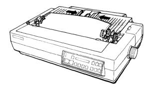
11. **Align** the pins of the pull tractor cover with the slots on the printer and attach the cover.
